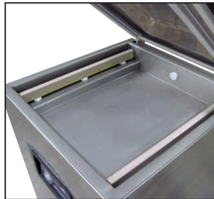
Two (2) 20" Seal Bars with Double Seal Wire
